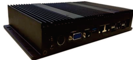
Side view: featuring Power, VGA, Serial, USB, LAN and CD ports
