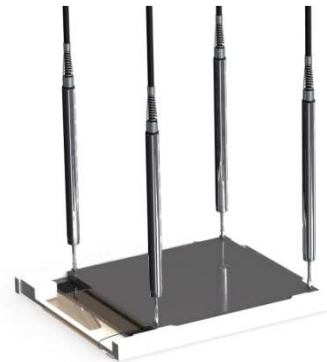
UFT checking a cell phone screen
