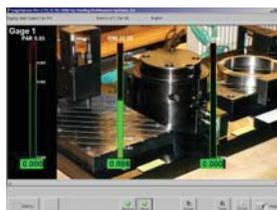
**Brilliant Graphics** Part status is displayed with the part image, bar columns, or digital readouts. Part images include importation of multimedia files such as photographs, CAD, TIF and more, including movies. The unique presentation provides a clear, easily understood operator interface reducing gaging time and errors.
