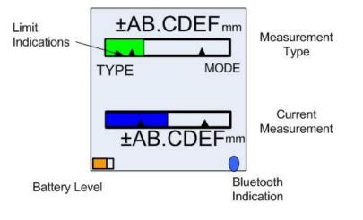
The display can be set to display the range and tolerance of the part being measured. (e.g. 28 ±0.05 mm)
